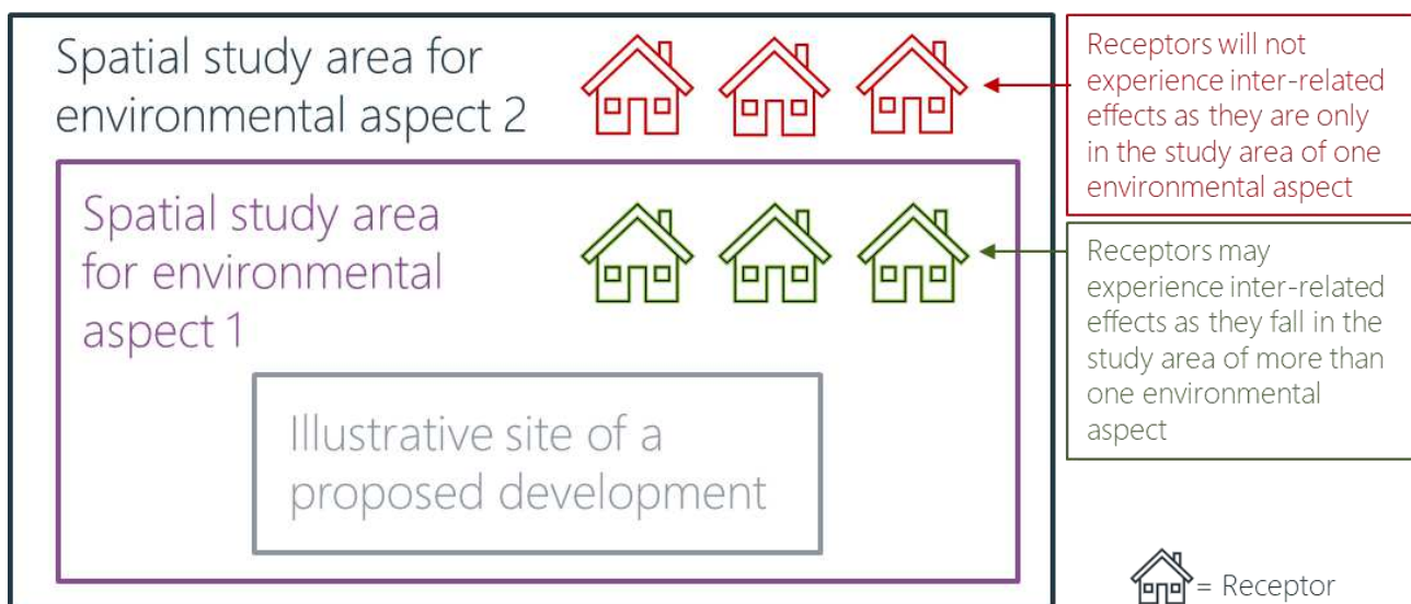
Graphic 177.1 Illustrative example of the spatial scope and study area for an example receptor
